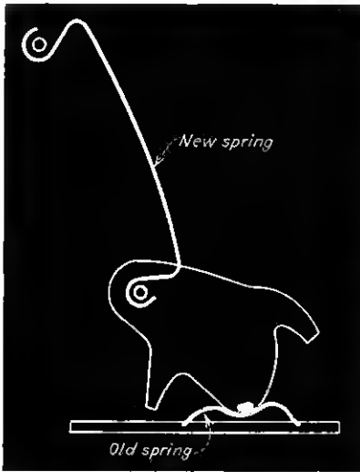
A new type of spring is available for Emerson models 397 and 374
